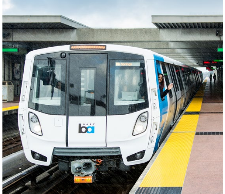
BART’s new train cars will feature three doors on each side to reduce noise, improve reliability and increase capacity.
