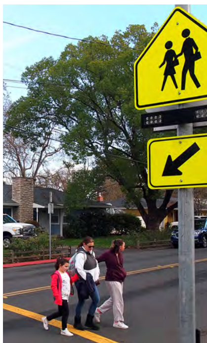
The Rapid Flashing Beacon (RRFB) - activated by pushing a button to alert on-coming vehicles. RRFB use provides higher visibility for pedestrians crossing a street
