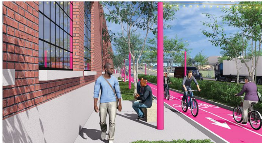
PLANTING BUFFER BETWEEN THE STREET WOULD NEED TO BE WIDENED, BIKE SURFACE TREATMENT AND FURNISHING WOULD BE NEW
