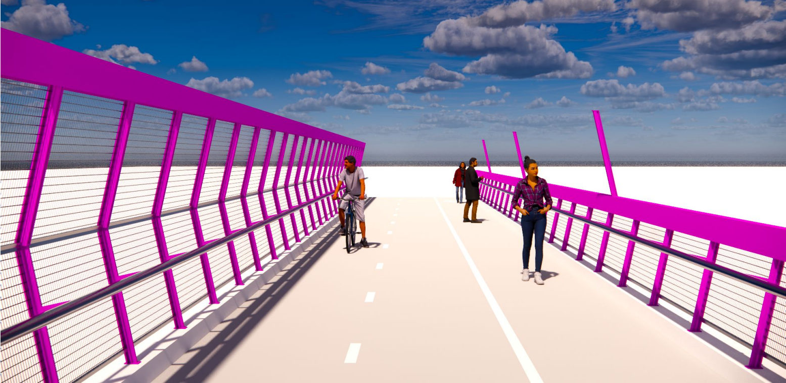
Painted top rail and post
