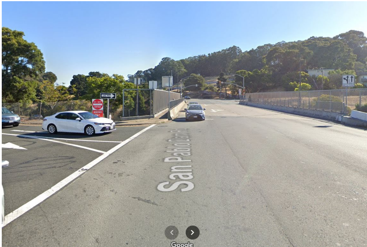
Figure 15. Looking east on SPDR at westbound I-80 off-ramp terminus; no crosswalk or bike lane striping is present on SPDR; 4-foot-wide sidewalk on north side of overcrossing visible in center left of photo. Photo credit: Google.
