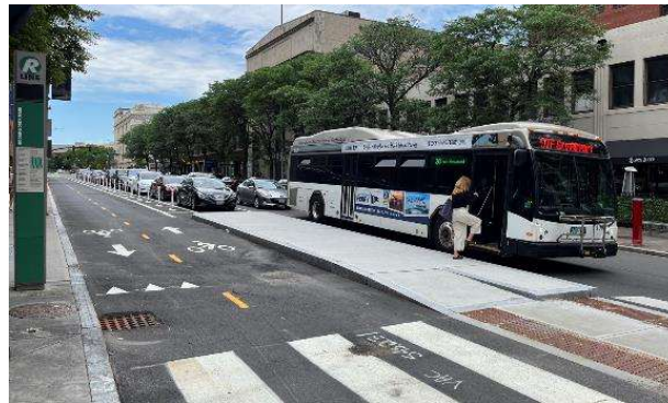
Left to right: In-lane bus stop adjacent to on-street parking, Floating bus stop in line with on-street parking, fully separated bike lane in dense mixed-use neighborhood. Source: Toole Design
