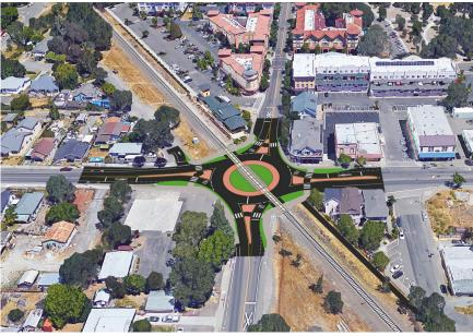
Roundabout Option – would replace existing traffic signal and railway safety improvements would be added
