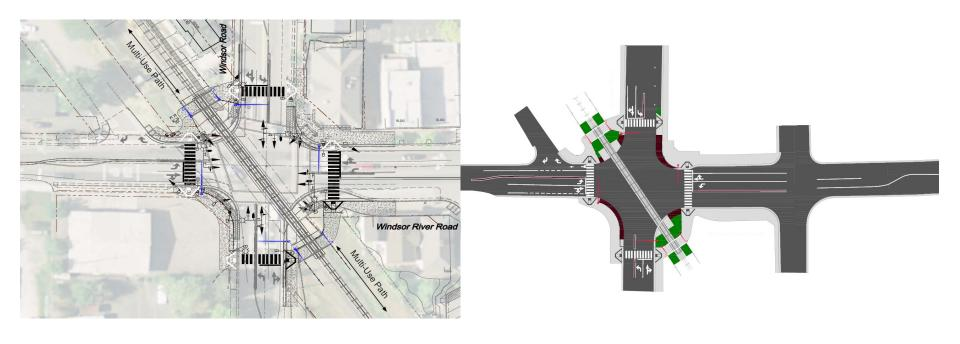
Traffic signal modification – would include signal and railroad gate relocations, median island extension, pedestrian controls, and sidewalk construction
