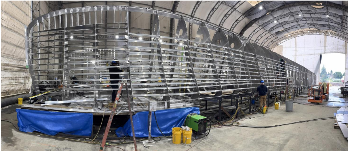
WETA 400 passenger electric ferry fabrication WETA Photo
