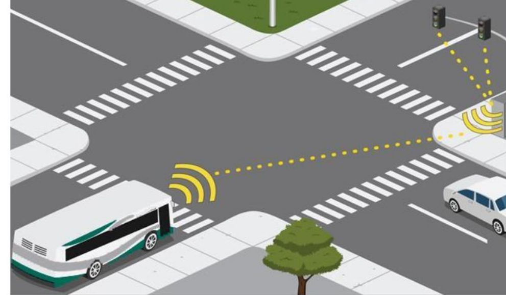
Figure 1: Transit Signal Priority (TSP) System
